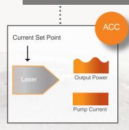
ACC (Automatic Current Control) mode is standard for all devices. The laser is controlled from diodes current set point.
